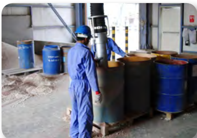
PURATEK® DSS Vacuum system in operation - sucking spent catalyst from barrels
