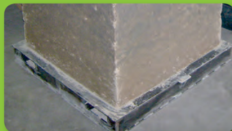
Ingots after removing of side walls
